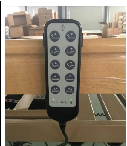
Hand Controller with conductive switch in case of wrong operation
